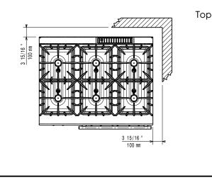
Gas Power:<br/>391013 (E9GCGL6C10)52.5 kWStandard gas delivery:<br/>Gas Type Option:<br/>Gas Inlet:Natural Gas G20 (20mbar)<br/>LPG;Natural Gas<br/>1/2"Key Information:Key Information:
